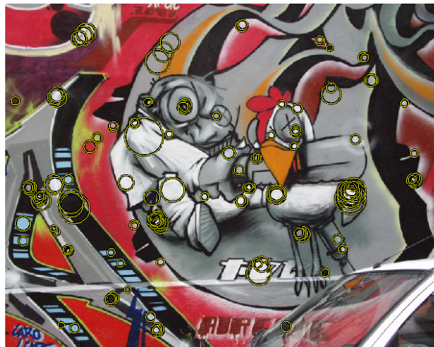
Fig. 4. The strongest responses of WaldBoost Hessian-Laplace region detector (similar number of responses as in Figure 3). \bar{T}_S = 1.68 .
