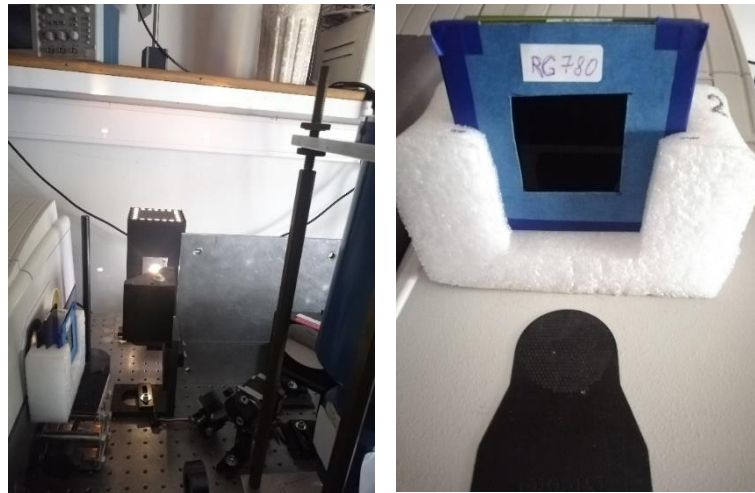
Figure 33 Front view of the measurement setup for FTPS and I-V measurement with 3 sun intensity light source Institute of Physics, Prague (left). Types of filters used for the experiment, Institute of Physics, Prague (right)
