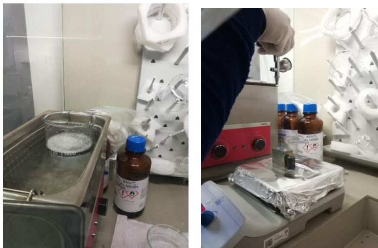
Figure 25 Cleaning by sonicating using acetone and ethanol (left). Spray pyrolysis for depositing TiO 2 layer (right).
