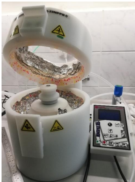
Figure 19 Spin Coating equipment from Laboratory of Department of Advanced Photovoltaics, FEL, CVUT
