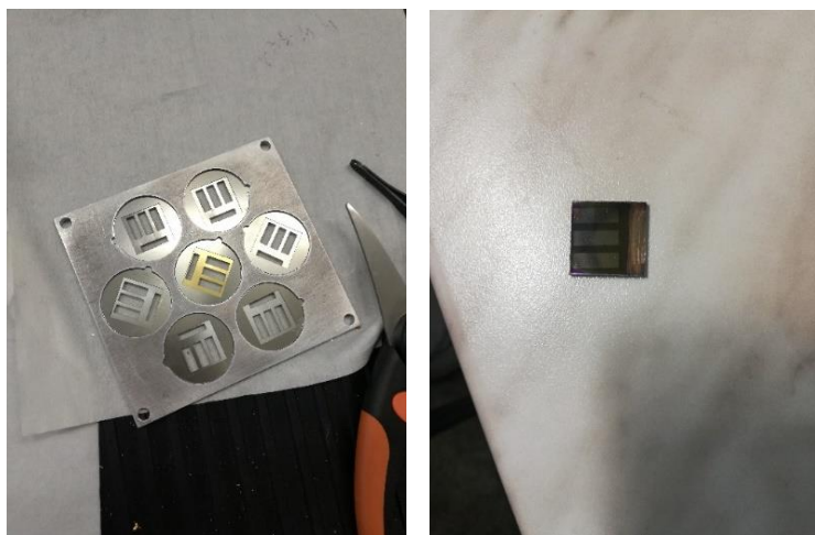
Figure 31 Shadow masking of solar cells with Au (left). Finished Perovskite Solar Cell (right).
