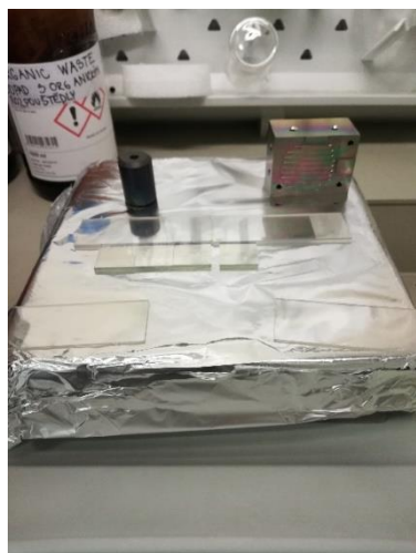
Figure 26 Substrates on hot plate to dry after deposition
