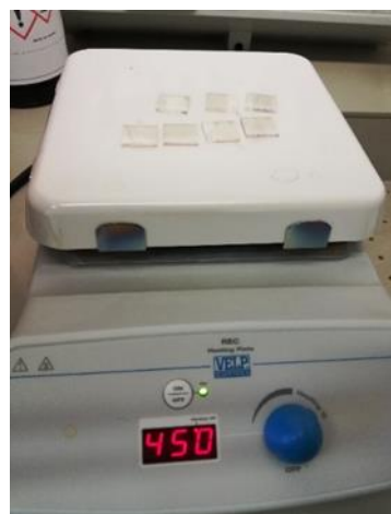
Figure 28 Deposition of M-TiO 2 using Spin Coating (left). Sintering of substrates at 450 °C for 30 minutes (right)
