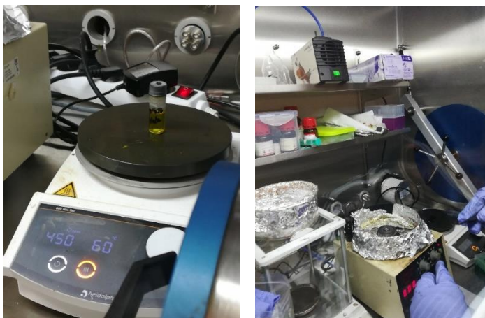
Figure 29 Magnetic stirring of perovskite solution (left). one step deposition of perovskite solution by spin coating (right)
