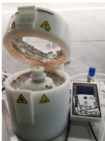
Figure 28 Deposition of M-TiO 2 using Spin Coating (left). Sintering of substrates at 450 °C for 30 minutes (right)
