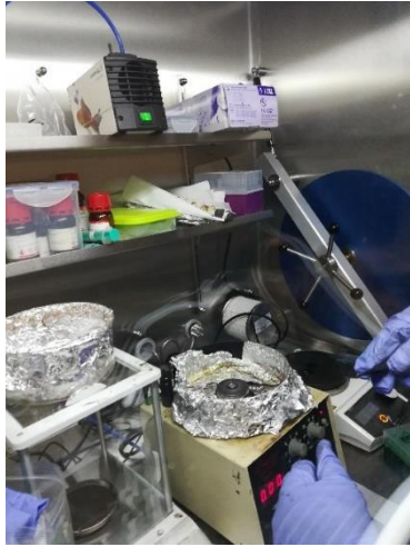
Figure 20 One step deposition by Spin Coating in Nitrogen glovebox at FEL, CVUT
