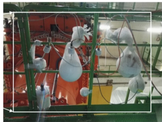
Figure 3.6: Photo of the Bonner sphere spectrometer during Run 2 in the CMS cavern [56].
