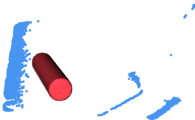
Figure 2.6: Very bad segmentation of detected object with outliers
