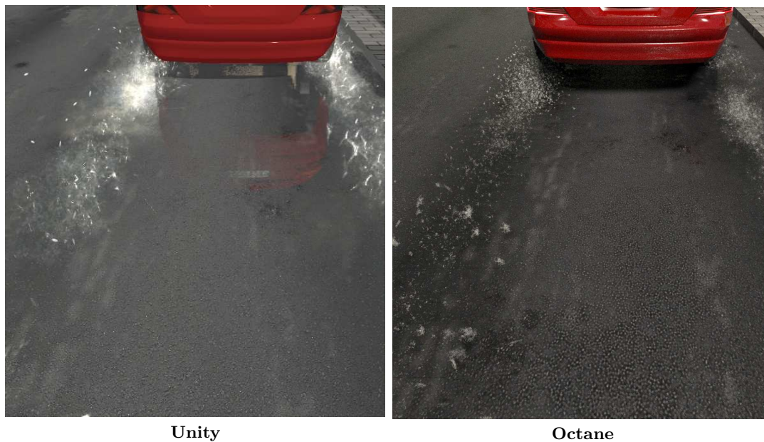
Figure 5.8: ( Unity ) The splashes projected from the bottom of tires are smooth and interact with light in a way that displays the specular glints of the water material. Part of the splash goes sideways (side waves), and the small particles in the air imitate the spraying of tiny drops. ( Octane ) The splashes rendered in Octane are opaque, better resembling the spraying particles behind the wheel.
