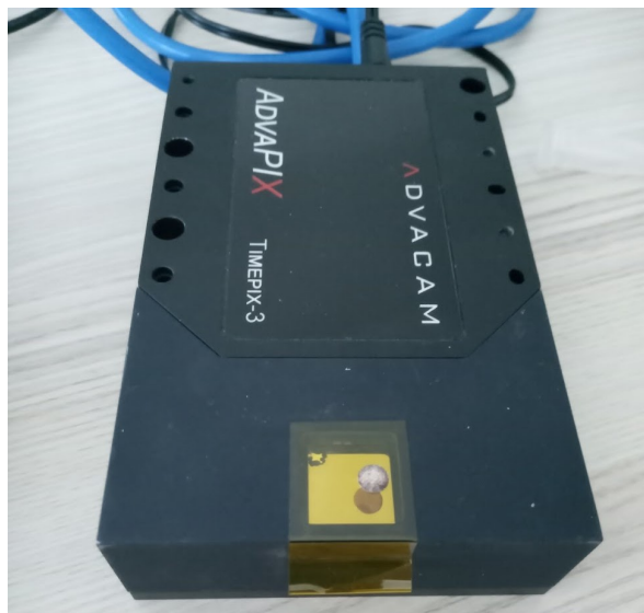
Figure 4.1: ADVAPIX TPX3 with Am241 source from smoke detector
