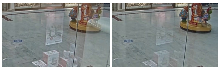
Figure 3.3: Image taken without a polarizer filter (left) and with polarizer filter (right).
