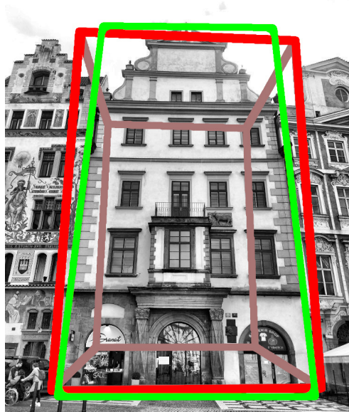
Figure 5.3: Possible gain of accuracy in case of improving reference images. The green quadrilateral is what has been detected and the red quadrilateral is the final product of a volume understanding. The difference between them is then the accuracy loss that was caused by having inaccurate reference images. Photo: author
