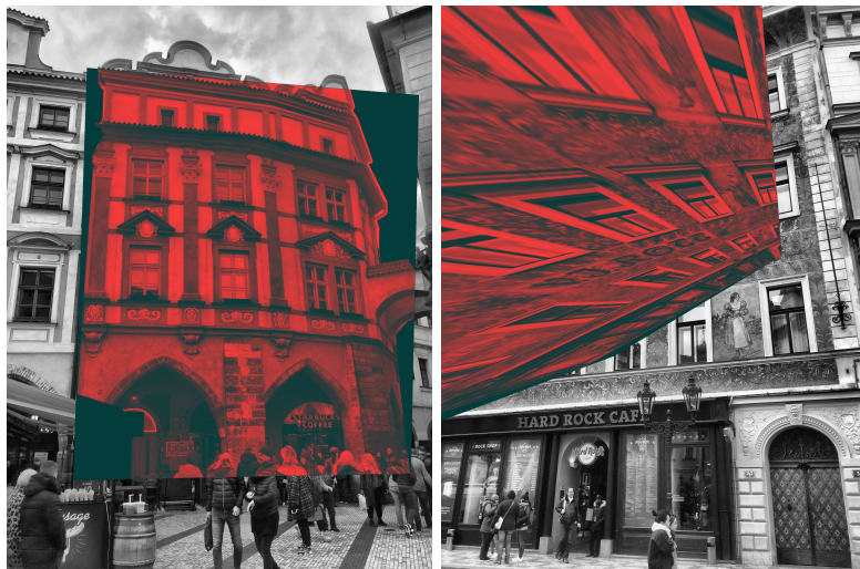
Figure 3.7: Early evaluation of our prototype. Correctly displayed object (building) in the scene on the left and badly displayed on the right. Building photos are from Jan Šefčík’s image database [1].
