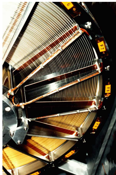
Figure 4.3: Close up of a mirror arrangement inside the X-ray telescope XMM-Newton. [48]
