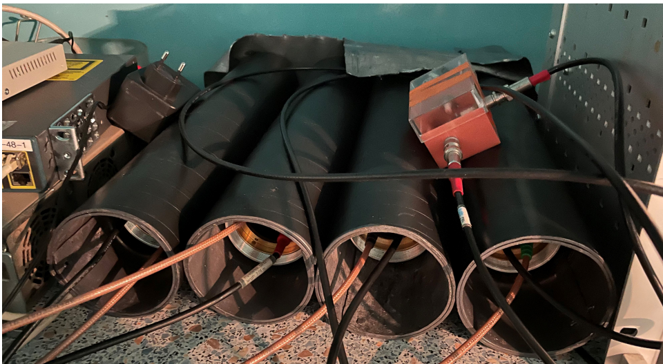
Figure 5.4: Setup of four scintillation detectors in a Faraday cage, numbered PM1-PM4 from the left.
