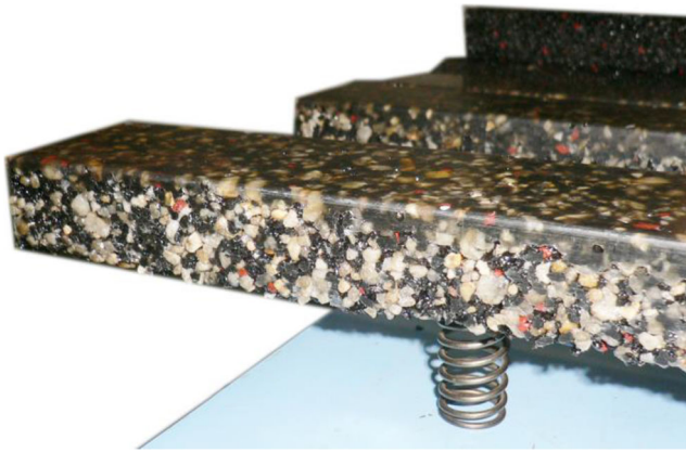
Fig. 20 Boundary conditions—beams on flexible springs
