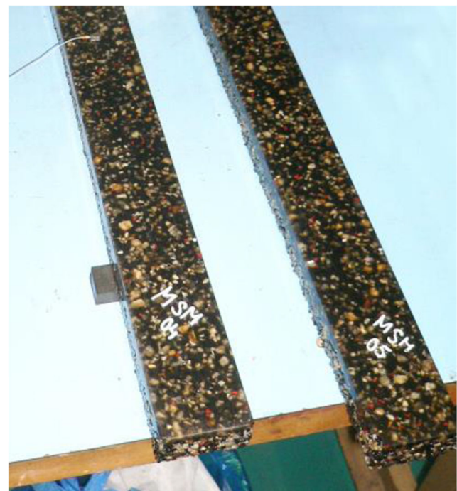
Fig. 19 Beam coupons made from particle composites
