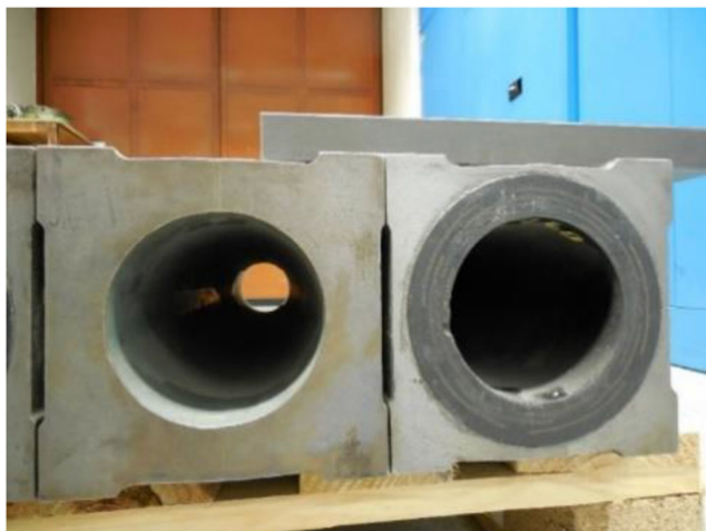
Fig. 9 Model hybrid spindle ram–reference cast iron ram (left), hybrid ram with reduced metal wall thickness and reinforcing composite tube (right)
