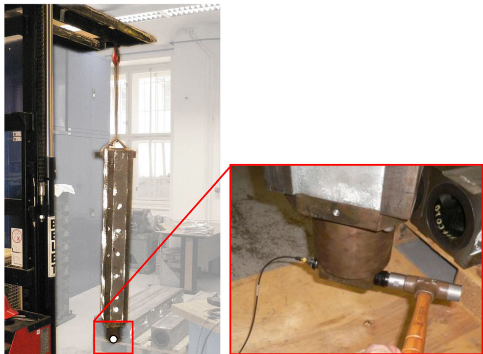
Fig. 10 Boundary conditions for model hybrid ram stand-alone testing. Detail of the excitation and response measurement on the right
