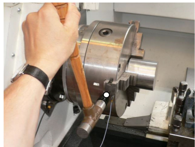
Fig. 34 Experimental modal analysis on lathe with hybrid spindle stock: excitation and response on the chuck
