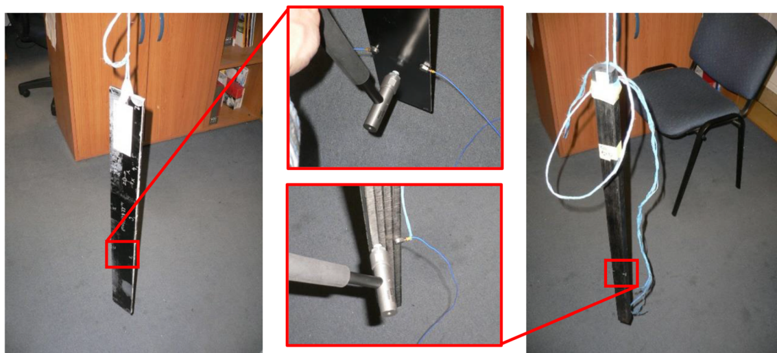
Fig. 5 Experimental modal analysis of 2D composite coupons (coupons #1–#7 on the left, #8–#10 on the right)
