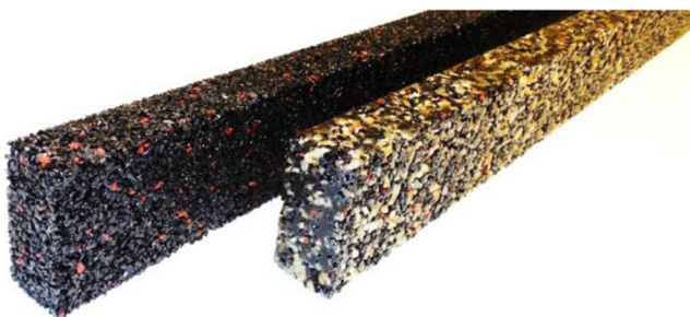
Fig. 3 Basic beams from particle composites (REC on the left, GREC on the right)
