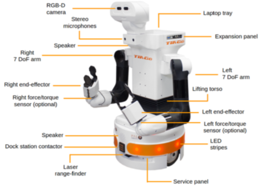
Figure 3.1: PAL Robotics TIAGo++ robot components [PALb]
