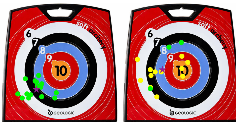
Figure 6.3: Target with arrow hits marked as green circles for stucked arrows and yellow circles for bounced arrows, distance 4 m (left) and 4.5 m (right) [bow]
