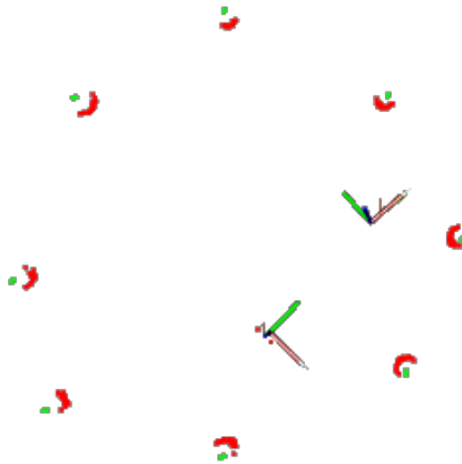
Figure 3.1: Red points are data from the laser scanner, whereas the green dot is the circle center estimation. Two agents are found in the center obtaining this obstacle laser scan.
