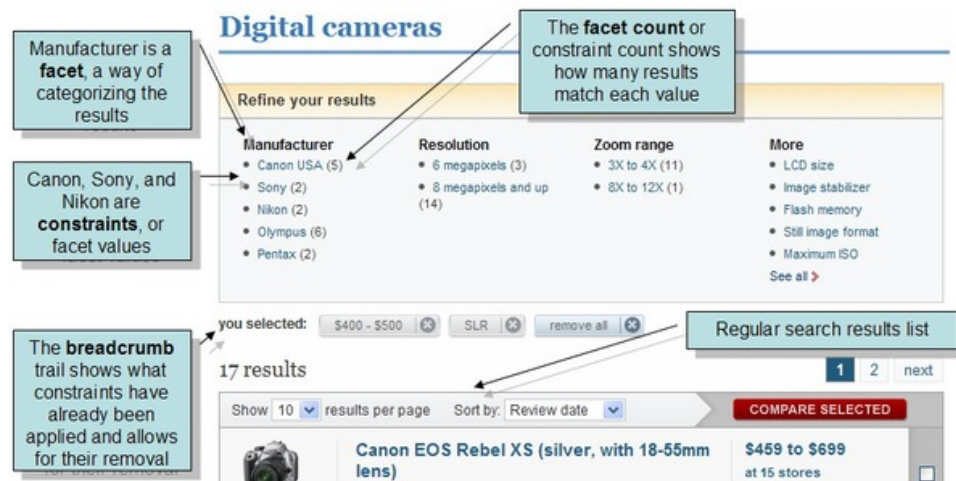
Figure 2.1: Demonstration of facet use in e-shops, where there are facets, their selection values and the number of searchable results for each value.
