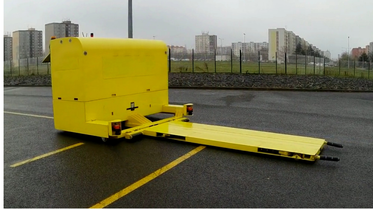
Figure 2: Prototype of the parking robot for which the Chronorobotics Laboratory develops the software and with which the data for experiments were collected.
