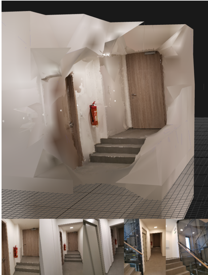
Figure 1.1: Reconstruction created with CR commercial software resulting in 5/23 registered images in this model.
