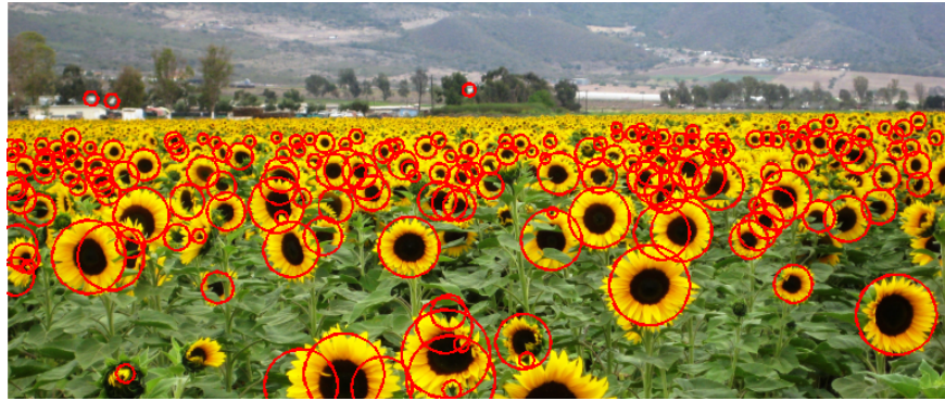
Figure 2.1: Detected blobs in sunflower image obtained by detecting Hessian maxima in scale-space. Image taken from [1].
