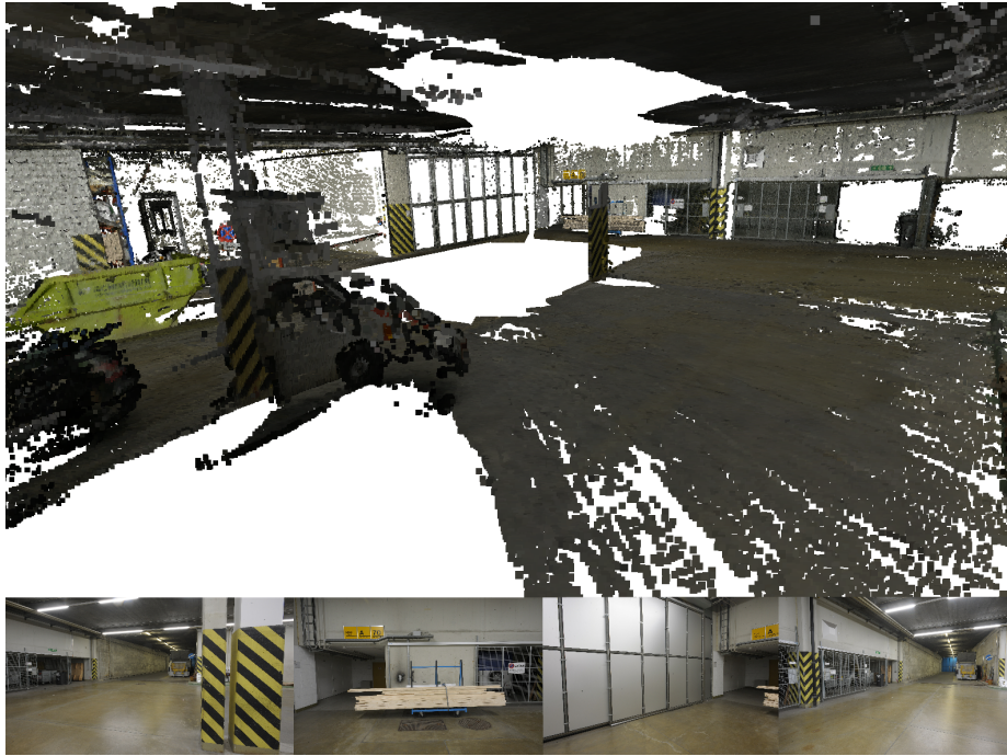
Figure 1.2: Example of environment, where are projects such as ARTWIN or SPRING applied. On the picture is the delivery area dataset from ETH3D datasets, which is then used in further comparisons. The dense reconstruction on the image was created with the baseline SIFT correspondence search combined with the COLMAP pipeline.
