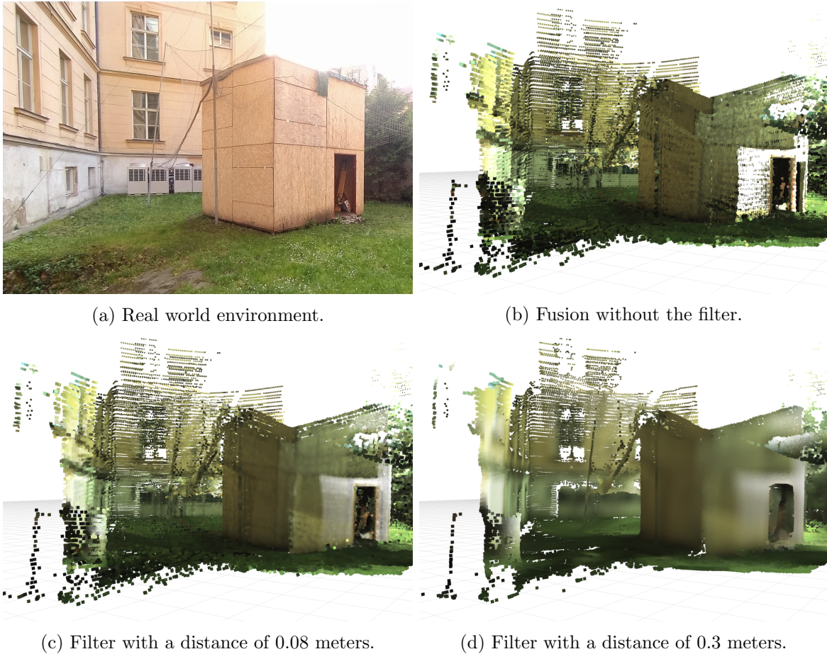
Figure 6.9: Comparison of the real-world environment and resulting point clouds with several setting of Gaussian kernel convolution filters.
