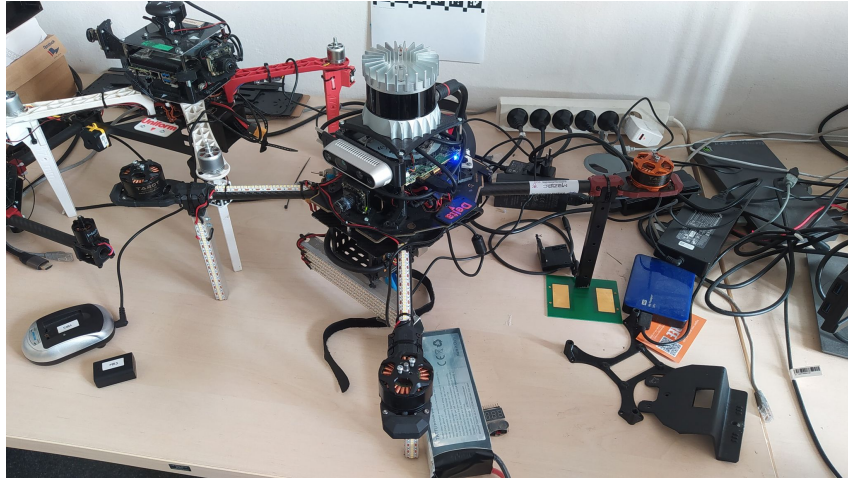
Figure 6.2: Camera-LiDAR setup on UAV.
