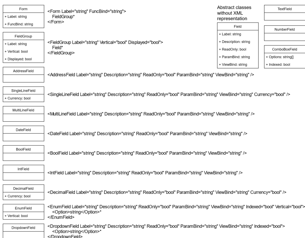
Figure 3.13: A mapping of the forms model into the XML syntax
