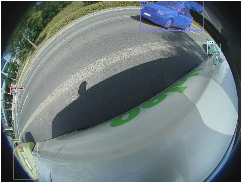
(a) Vignetting on the left side and reflection causing errors for detection on the blue car
