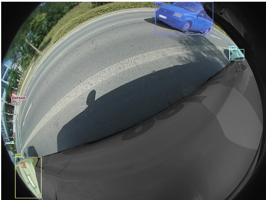
(b) Masked area displayed with monochrome filter suppressing aberrations
