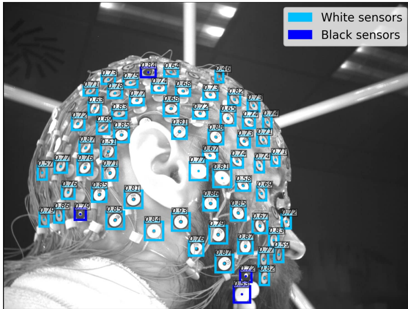
Figure 4.7: Example of the Template Matching output with match score of each bounding box
