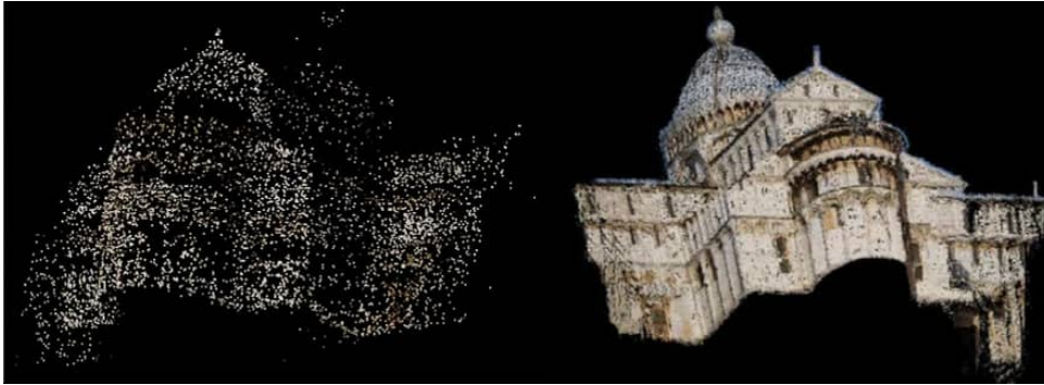
Figure 2.9: Illustration of sparse (left) and dense (right) 3D reconstruction [27]
