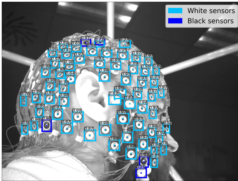
Figure 4.4: Example of the Faster R-CNN output with confidence score of each predicted bounding box
