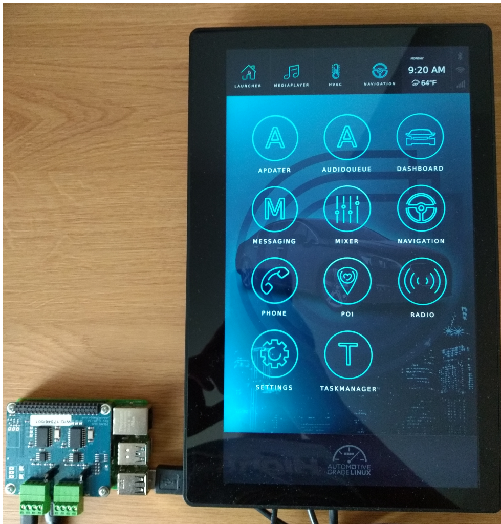
Figure 3.2: Showcase platform: Automotive Grade Linux running on Raspberry Pi 4 with WaveShare touchscreen connected
