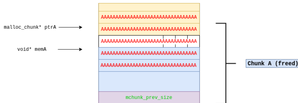
Figure 2.9: Illustration of heap memory corruption caused by overflow
