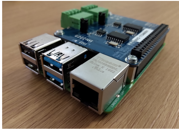
Figure 3.1: Showcase platform: Raspberry Pi 4 with PiCAN 2 DUO extension board attached
