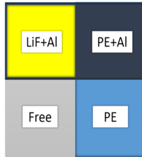
Figure 1.2: Schematics of converter layout in a TPX device. [7, Figure 1(b)]
