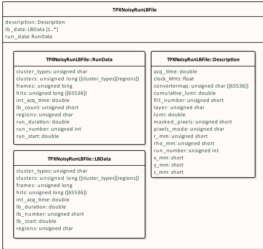
Figure 3.8: Structure diagram of a TPX LB file before noisy pixel removal.
