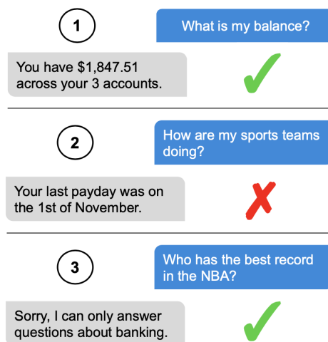
Figure 1.1. Example of interaction between user (right side) and chatbot (left side). (1) – the user asks a question that belongs to an ID intent. (2) – the chatbot fails to detect OOD. (3) – the chatbot succeeds in the task, giving a fallback response [5].
