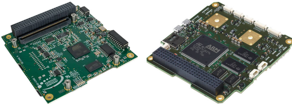
Figure 2.4. Photos of existing professionally developed OBCs. iOBC by ISIS (left) and SatBus 3C2 by NanoAvionics (right). Sources: ISIS, NanoAvionics.
