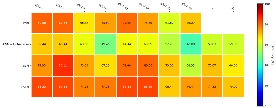
Figure 4.1: qb Soft Hand – Overview of classification performance over datasets. Performance of different classifiers is in rows, with increasing complexity of the classifier from top to bottom. Different datasets used are in columns. Please note, that “s” means “squeeze” and “sq” means “squeeze and release” datasets.
