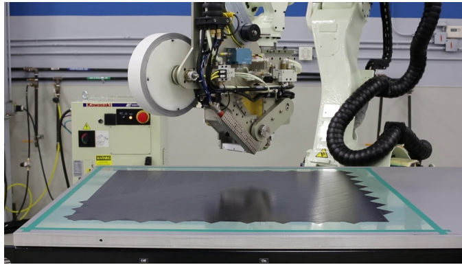
Figure 3.2: Prepeg tape laying head on a robot arm (white structure) [6]
