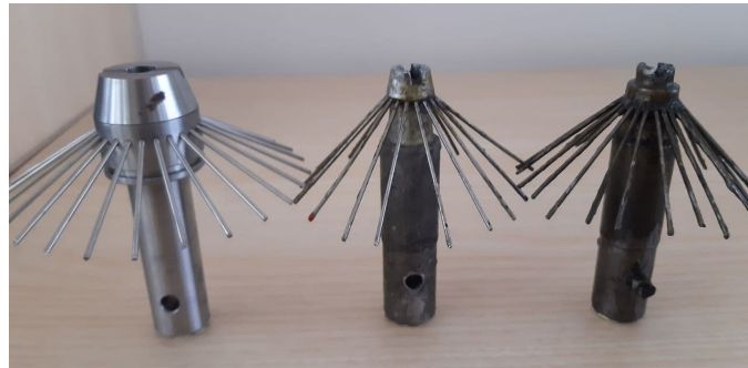
Figure 4.2: New and shiny pin holder (left), slightly used pin holder (middle), heavily used pin holder (right)
