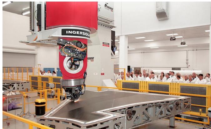
Figure 3.6: Ingersoll Mongoose fiber laying system [11]
