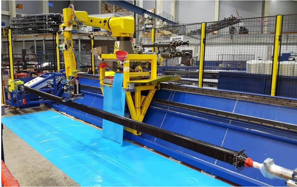
Figure 3.8: CompoTech RAFL (Robot assisted fiber laying) system where FANUC robot arm (upper yellow part) is laying carbon fiber on to the mandrel (black tube under the robot arm)
