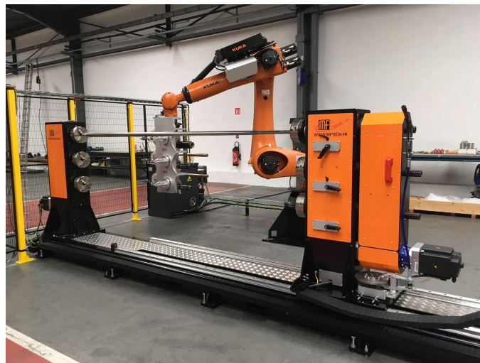
Figure 3.7: MF Tech system for standard filament winding [13]
