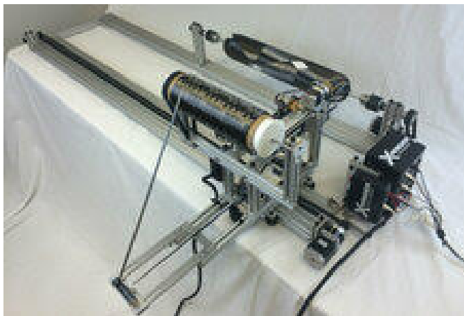
Figure 3.9: 4 axis filament winding machine X-winder [14]
