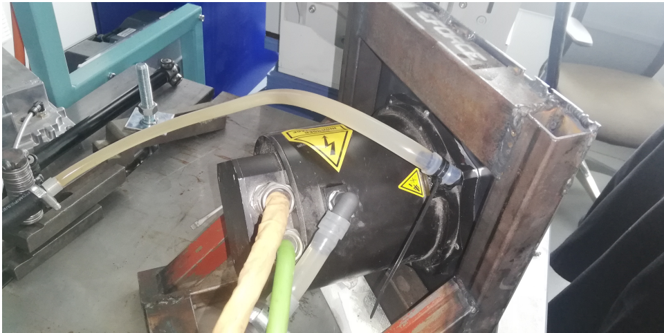
Figure 2.7: TG drives PMSM on the testing stand, during the testing
