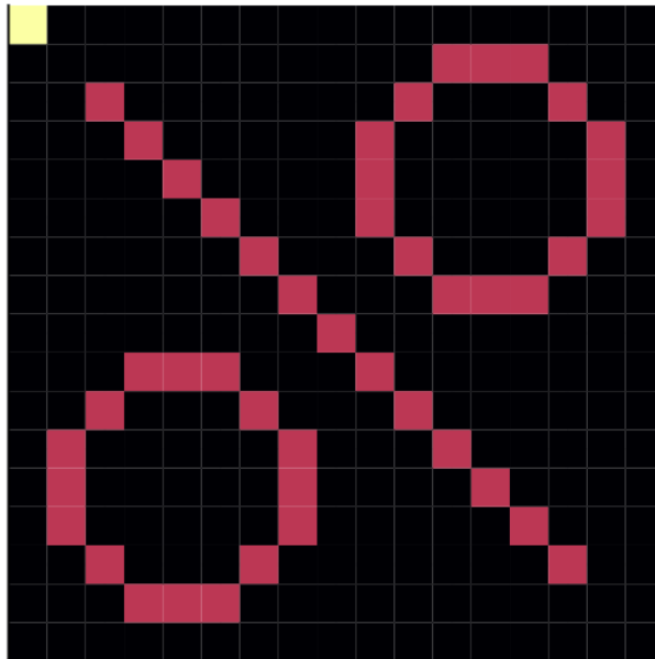
Figure 3.7: Example of a problem defined in the representation for neural network. Black squares are empty, red squares represent the image that needs to be painted and the yellow squares represent a robot. The goal is to paint a percentage symbol with robot starting at position (1,1)
