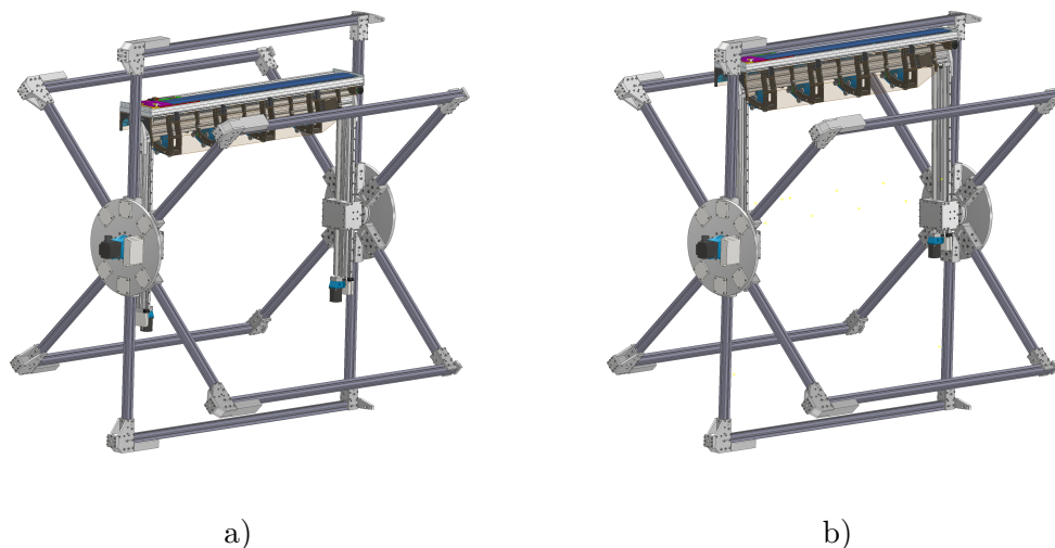
Figure 2.7. Example of the robot movement in the radial direction. On the figure a) is the robot in its default position. On the figure b) is the robot arm fully extended.
