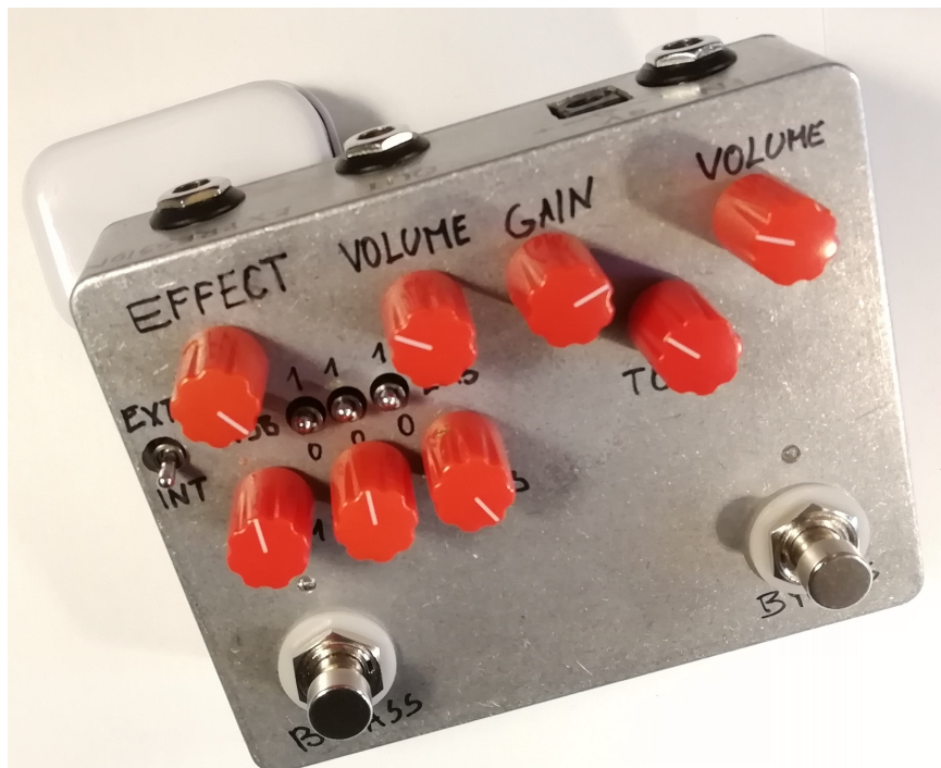
Figure 8.6: Angled top view of the fully assembled digital guitar pedal in enclosure with True bypass switching.
