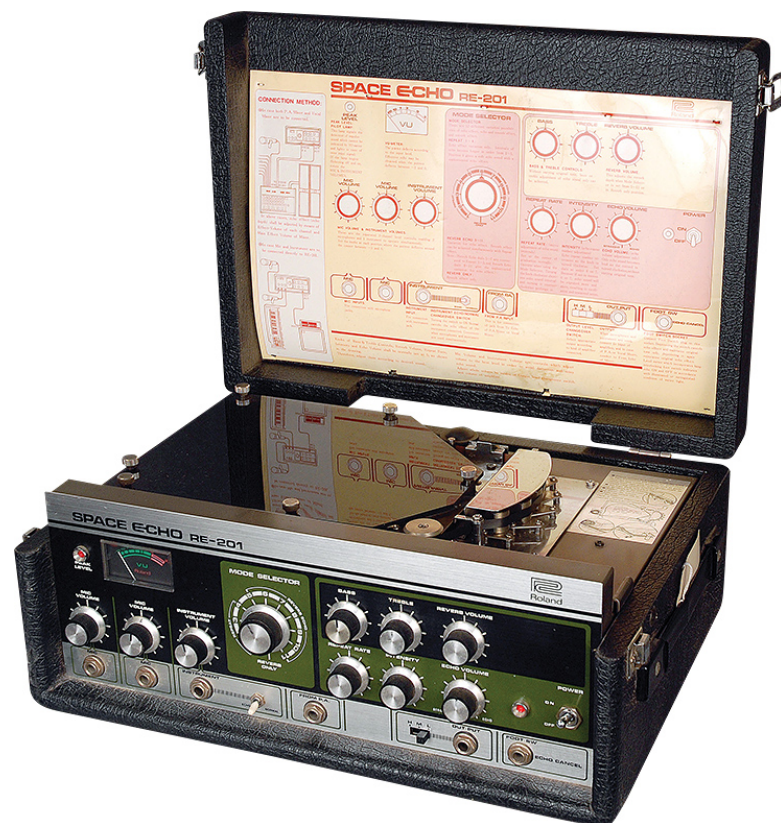
Figure 2.5: Example of a tape echo - Roland RE-201 Space Echo.[1]
