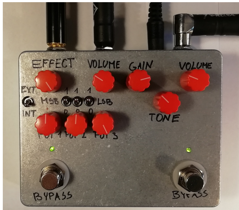
Figure 8.5: Top view of the fully assembled digital guitar pedal in enclosure with true bypass switching connected to signal chain.
