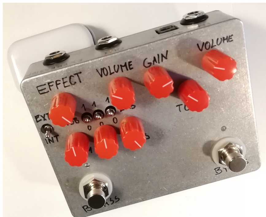
Figure 1.2: Angled top view of the fully assembled digital guitar pedal in enclosure with True bypass switching.
