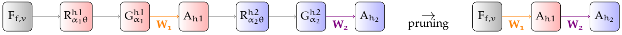
Figure 16: Demonstration of the pruning technique on a sample MLP model unfolded from a 2-rule template of \alpha_1 = \mathbf{W}_1 :: h_1 :- f. and \alpha_2 = \mathbf{W}_2 :: h_2 :- h_1.
