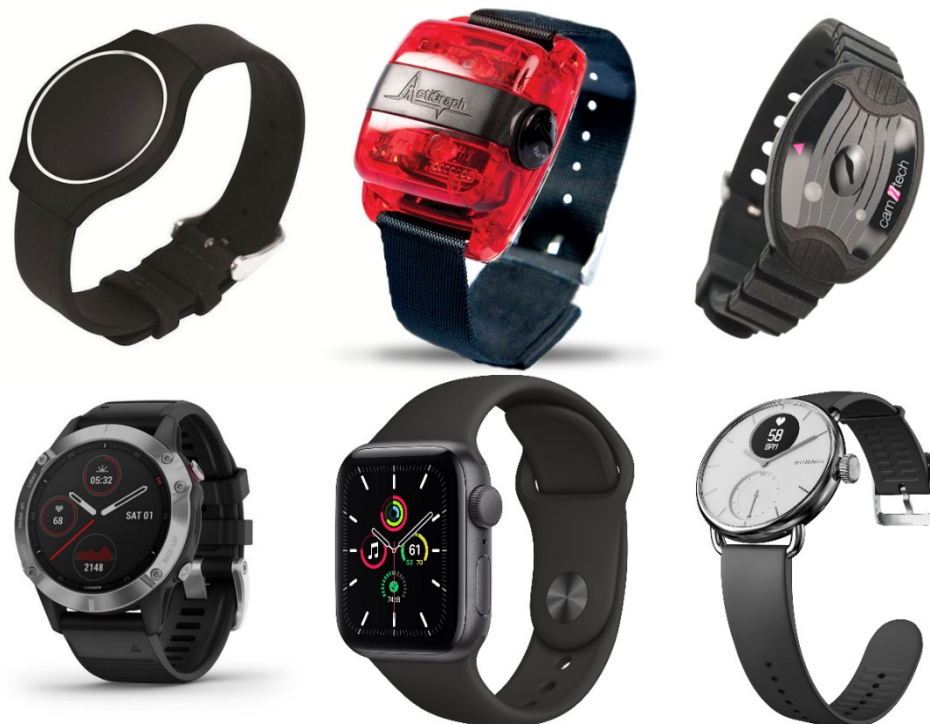
Figure 3.2 - Example of activity monitoring devices. In the upper row are presented the research wearables (MindG, ActiGraph, MotionWatch), which provide raw data for future analyses. In the bottom row are presented commercial smartwatches (Garmin, Apple, Withings). 7
