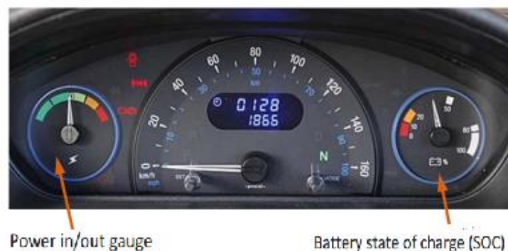
Figure 15 Analog gauges dashboard with SoC and Power in/out gauge
