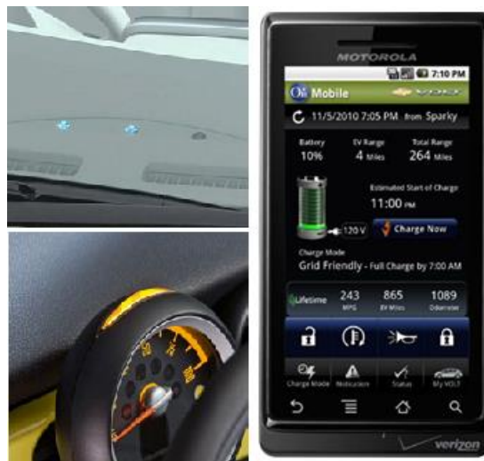
Figure 19 Top left Nissan leaf Charging indicator/ lower left MINI indicator/ right VOLT mobile application
