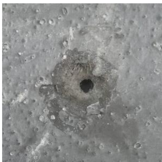
Obr. 79 Perforace UHPFRC desky projektilem [111].
