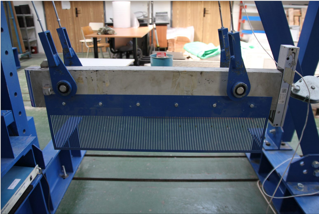
Figure 48: The impactor's attachment for interacting with the optical gate.
