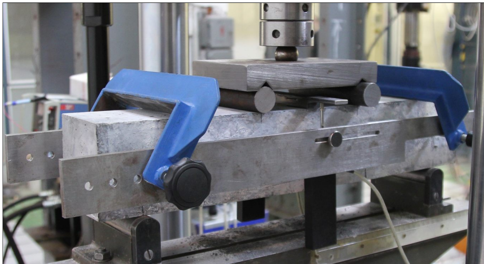
Figure 20: A typical four-point bending setup [21].
