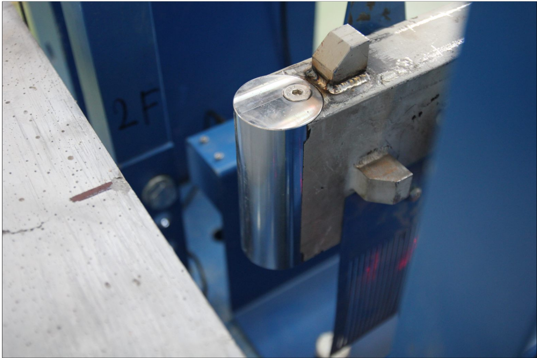
Figure 39: The detachable hardened nose of the impactor.
