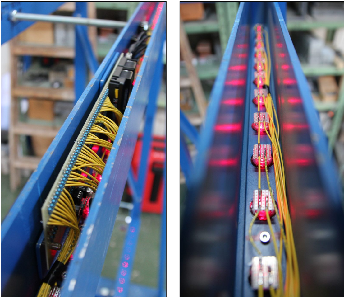
Figure 50: The photodiode circuitry in the top beam of the measuring frame.
