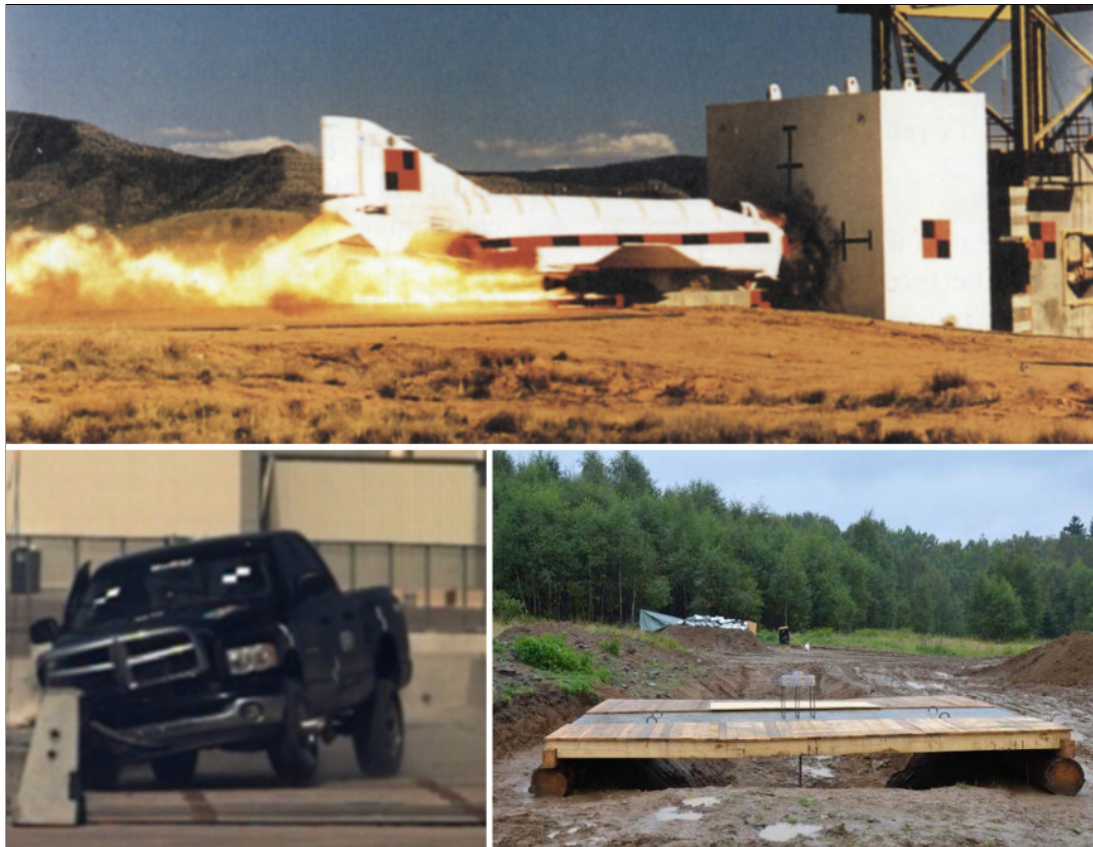
Figure 32: Examples of full-scale experiments. From the top-left plane-crash [84] car-barrier testing [85] blast loading of a concrete panel [86].
