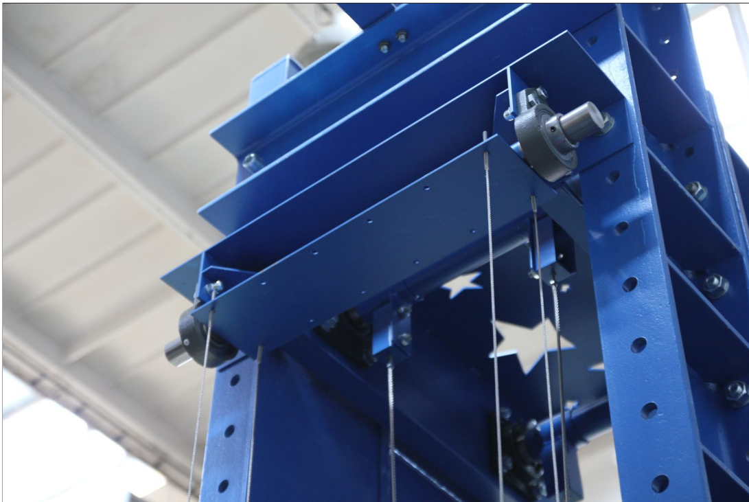
Figure 41: The mechanism that allows rotation of the specimen suspension.
