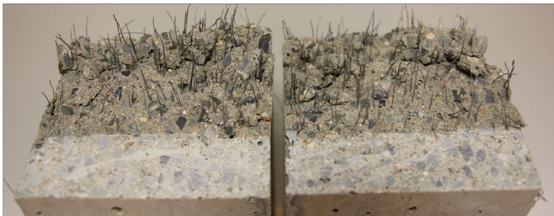
Figure C.1: Damage patterns after impact loading. Mixture HSC.
