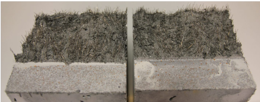
Figure C.5: Damage patterns after impact loading. Mixture R.
