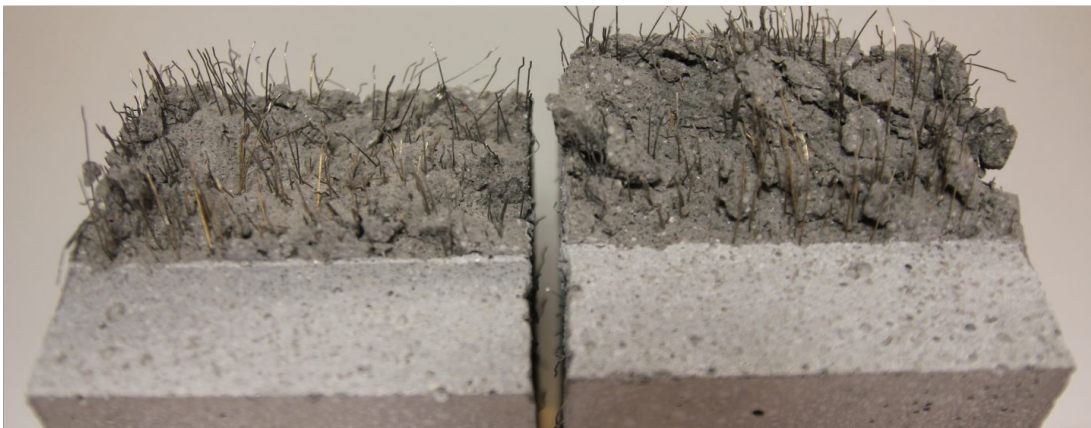
Figure C.3: Damage patterns after impact loading. Mixture DM.
