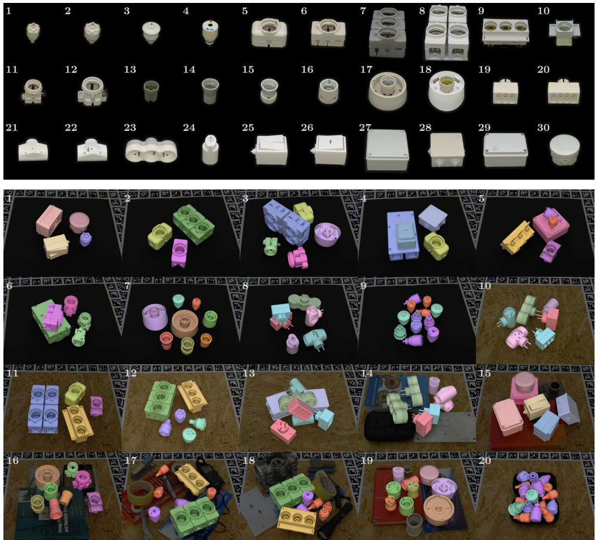
Figure 6.2. T-LESS objects and scenes. The dataset includes 3D models and training images of 30 objects (top) and test images of 20 scenes (bottom) – shown overlaid with colored 3D object models in the ground truth poses. The images were captured from a systematically sampled view sphere around an object/scene and are annotated with accurate ground-truth 6D poses of all instances of the modeled objects. Some objects are a composition of others. For example, objects 7 and 8 are built up from object 6, object 9 is made of three copies of object 10, and the center part of objects 17 and 18 is nearly identical to object 13.
