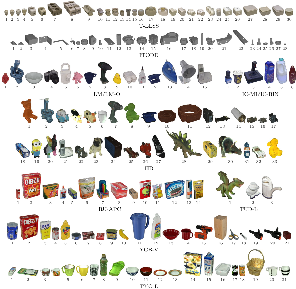
Figure 7.1. 3D object models available in the BOP datasets. The models are provided as 3D meshes with surface normal vectors and surface color. The color is saved per mesh vertex or as an UV texture. The models were created manually in CAD software or by KinectFusion-like systems for 3D surface reconstruction [178]. T-LESS includes both CAD and reconstructed models with surface color available only for the reconstructed models shown above. ITODD includes only CAD models with no color. The figure shows models rendered at the same distance.
