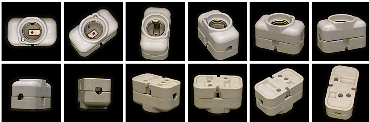
Figure 3.3. RGB channels of sample templates from [102]. Each object is represented by multiple (usually several thousands) templates showing the object under different 3D orientations (i.e., under different azimuth, elevation and in-plane rotation angles).
