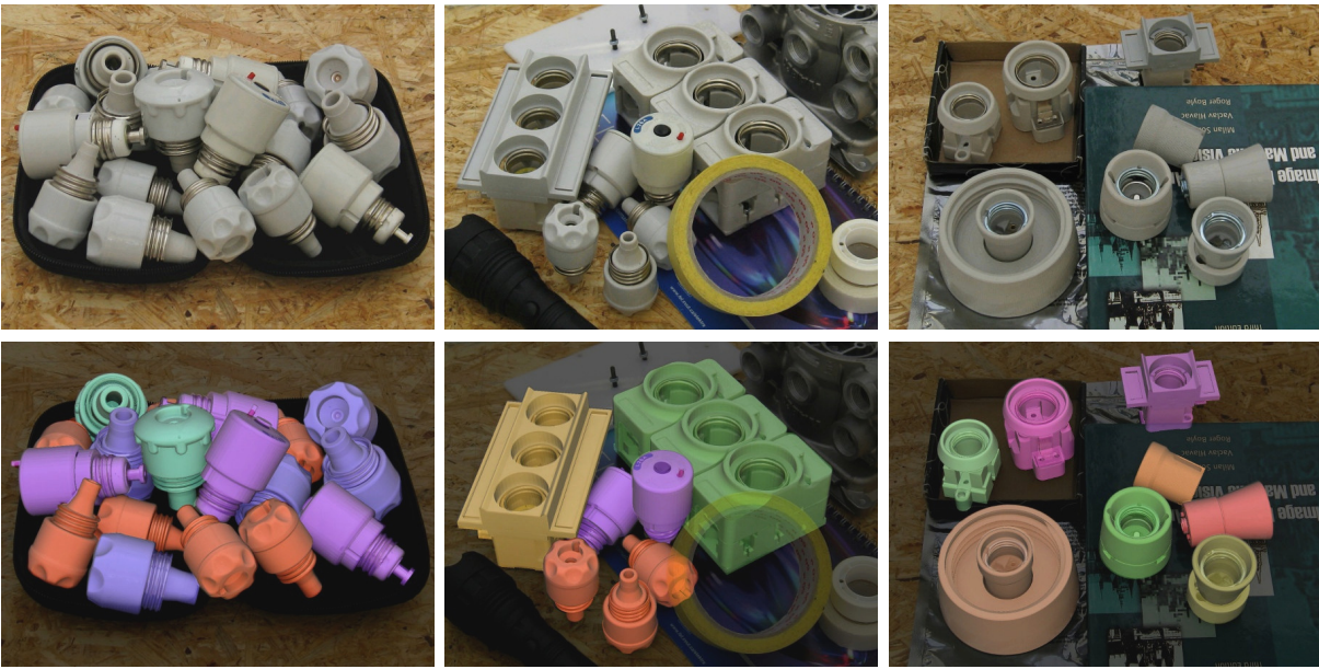
Figure 6.1. Challenges in T-LESS. Recognizing and estimating the 6D pose of T-LESS objects is challenging because the objects are texture-less, without a discriminative color, exhibit symmetries and similarities in shape and size, and are often seen under heavy occlusion and clutter. Cropped test images (top) are shown overlaid with colored 3D object models in the ground-truth 6D poses (bottom). Instances of the same object have the same color.
