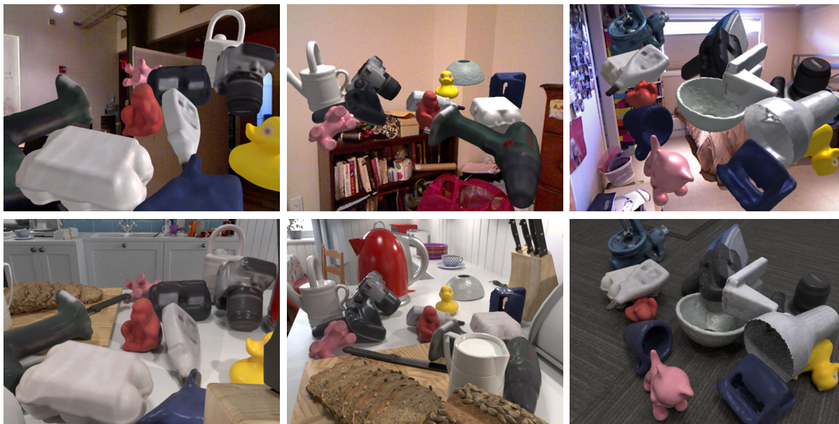
Figure 5.4. Types of training images. The baseline “render & paste” training images (top) were generated by rendering the 3D object models in the same poses as in the PBR images (bottom) and pasting the renderings on top of random photographs.
