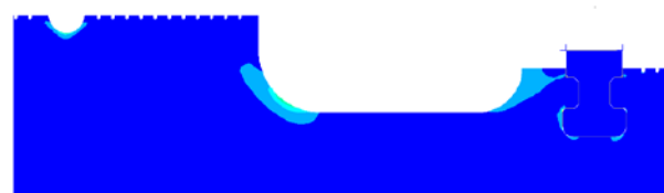
Fig. 10. Distribution of the fatigue damage computed by the Nihei method.
