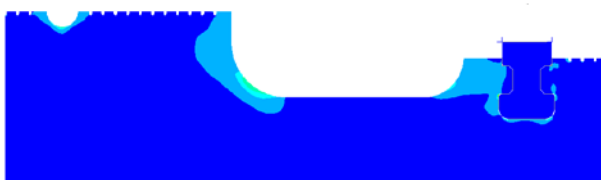
Fig. 9. Distribution of the fatigue damage computed by the SWT method.
