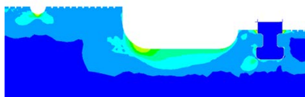
Fig. 8. Distribution of the fatigue damage computed by the DOA.
