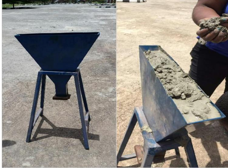
FIGURE 3. V-funnel apparatus and execution of V-funnel test.
