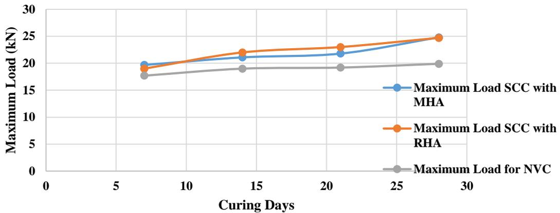
FIGURE 8. Plot of maximum load of SCC with MHA, RHA and NVC against curing days.
