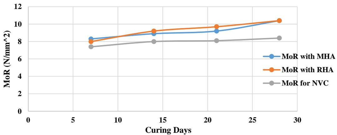
FIGURE 9. Plot of MoR for SCC with MHA, RHA and NVC against curing days.
