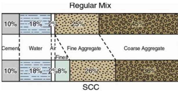
FIGURE 1. Materials proportion used in regular concrete and self-compacting concrete by absolute volume [6].
