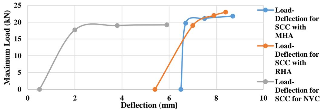
FIGURE 10. Plot of maximum load against deflection for SCC with MHA, RHA and NVC.
