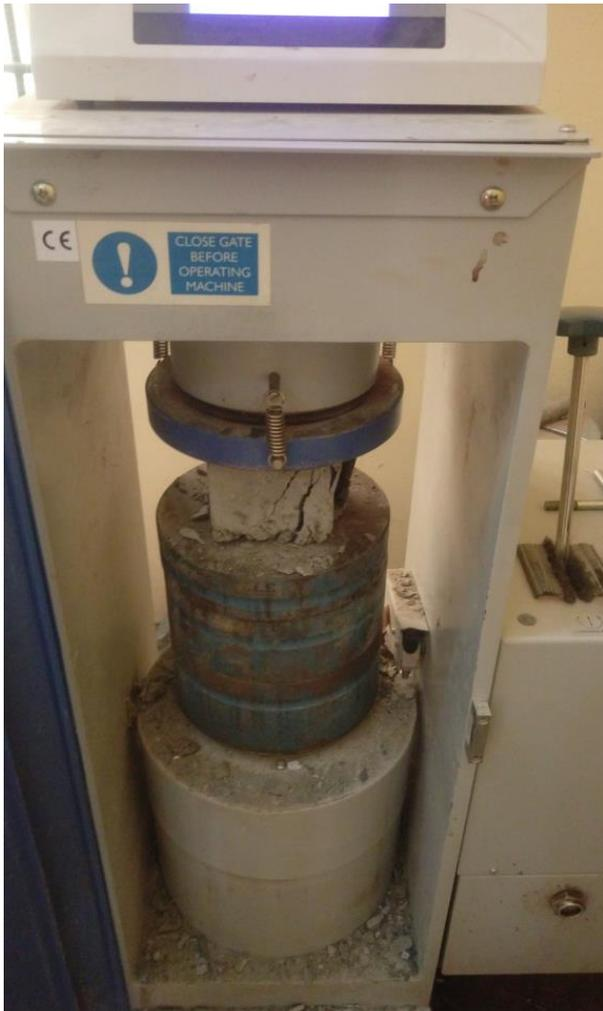
FIGURE 5. Crushing of concrete cube specimen.
