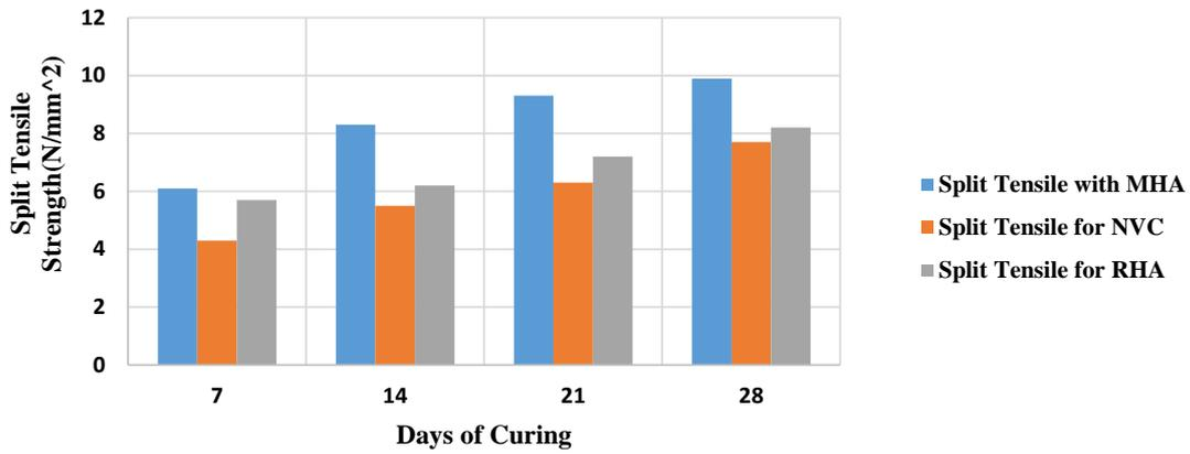
FIGURE 7. Variation of split tensile strength of SCC with MHA, RHA and NVC at grade M70.
