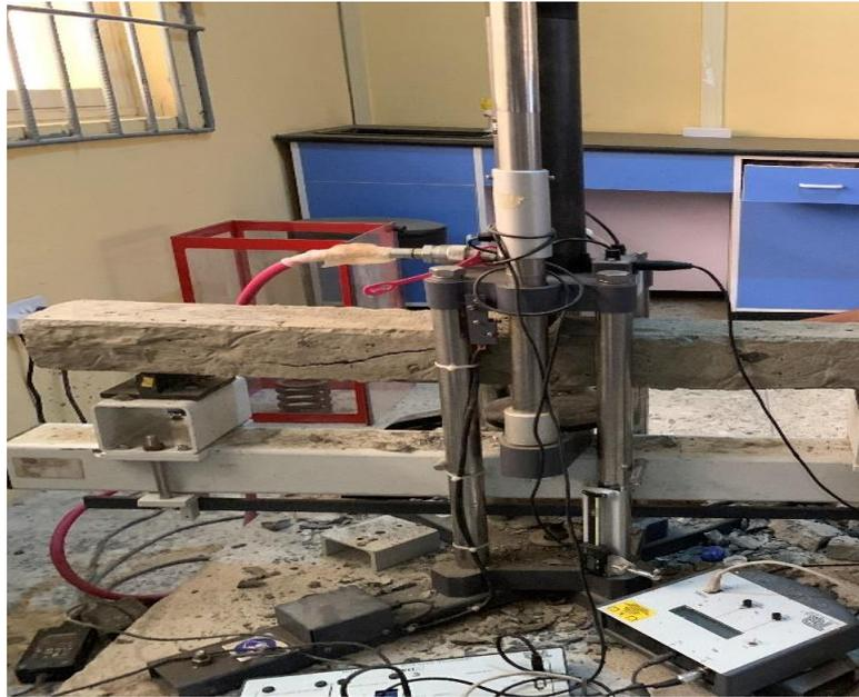
FIGURE 6. Flexural strength test of beam specimen using 100 kN-UTM.
