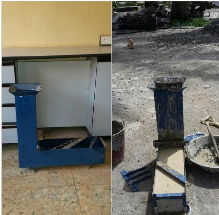
FIGURE 4. L-box apparatus and execution of L-box test.
