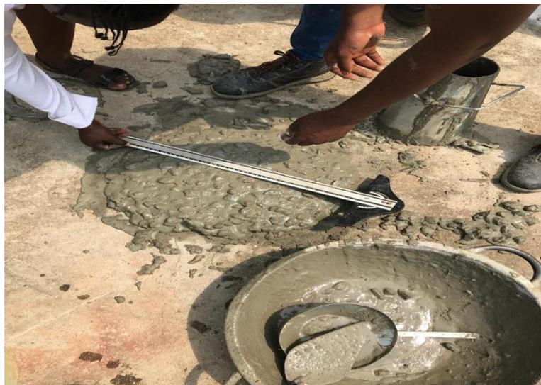
FIGURE 2. Slump flow measurement of SCC.
