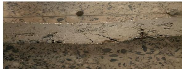
FIGURE 11. Crack pattern of reinforced concrete beam with EPS as replacement aggregate.
