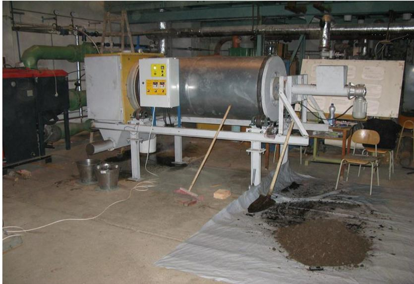
FIGURE 1. Experimental indirect dryer.
