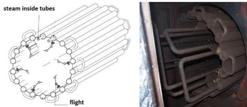
FIGURE 2. Steam heated rotary drum.
