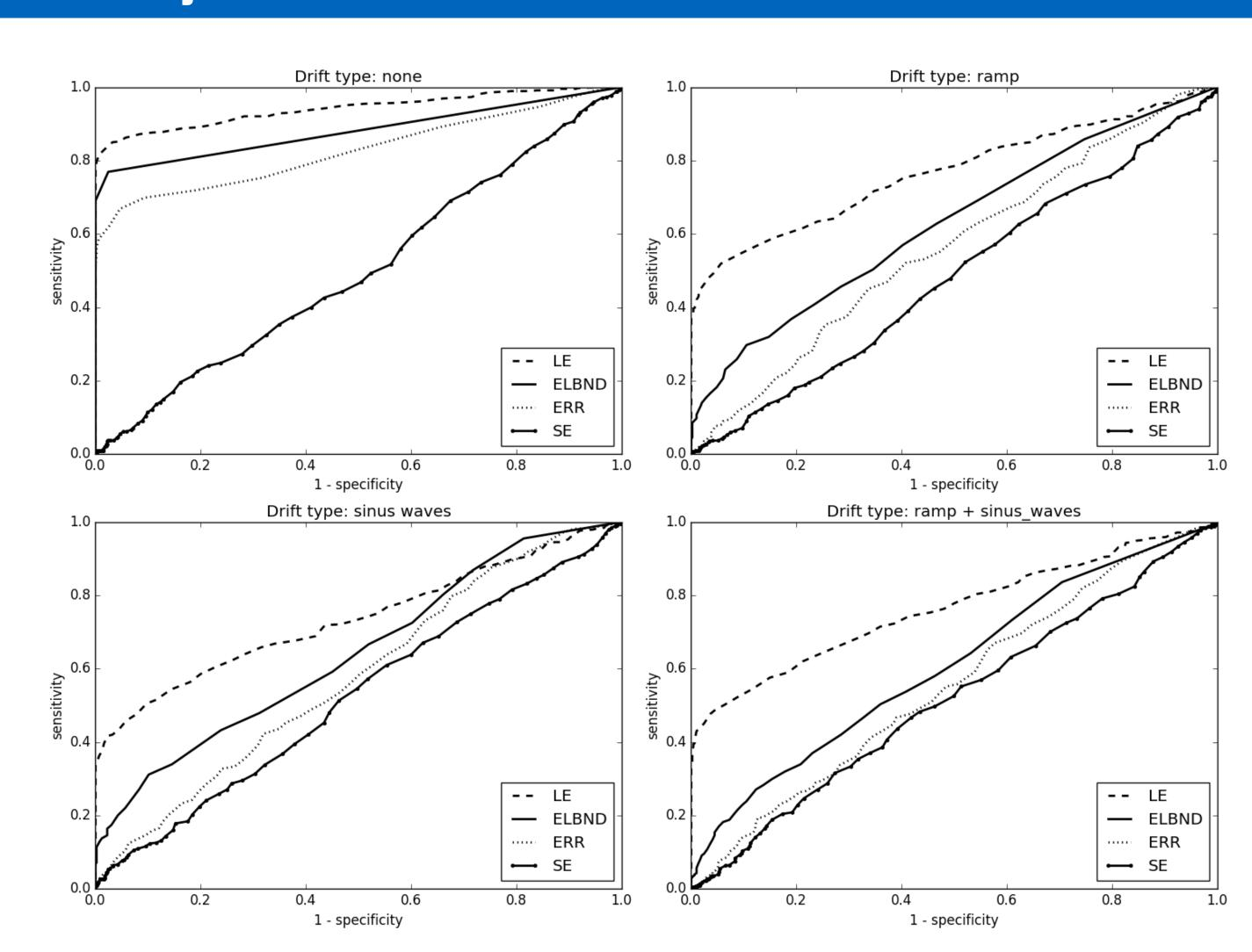
The ELBND method was tested with various types of non-stationary data with concept-drift and different types of noise [2,4]. Figure above shows that ELBND method can compete and in some cases even overcome other state of the art methods - Learning Entropy (LE), Sample Entropy (SE).
