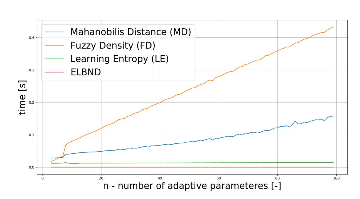
According to the Table and Figure above [3], the ELBND method is suitable for online use and can be considered fast in comparison with similar methods.
