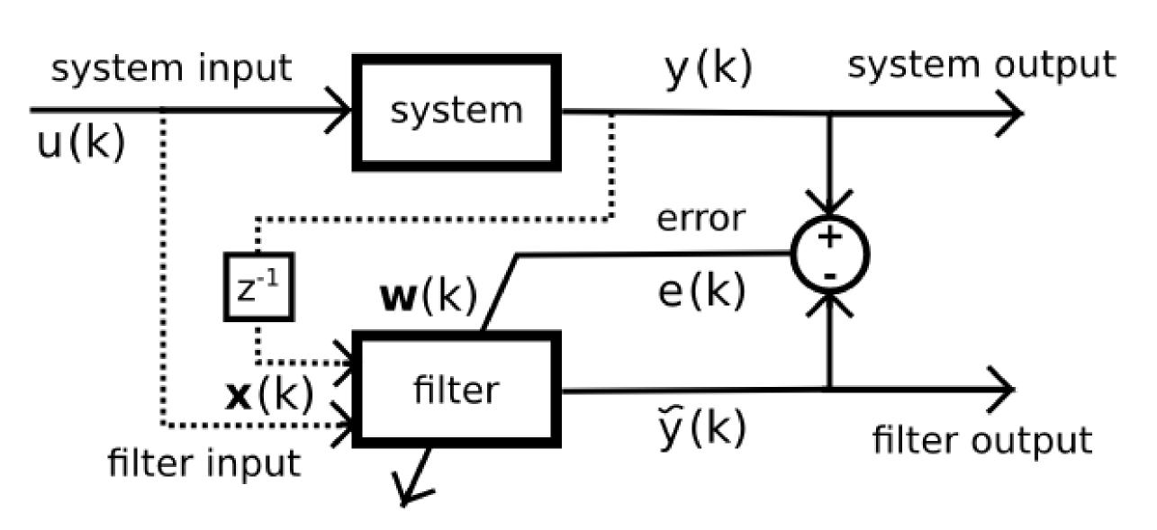
This prediction setup is suitable for online use. Many different adaptive algorithms can be used in the adaptive filter via ELBND method novelty detection, for example: LMS, NLMS, RLS, GNGD [1-4].
