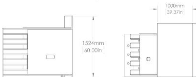
Figure 3 Flat 150 Barrier, Side and Front Views
