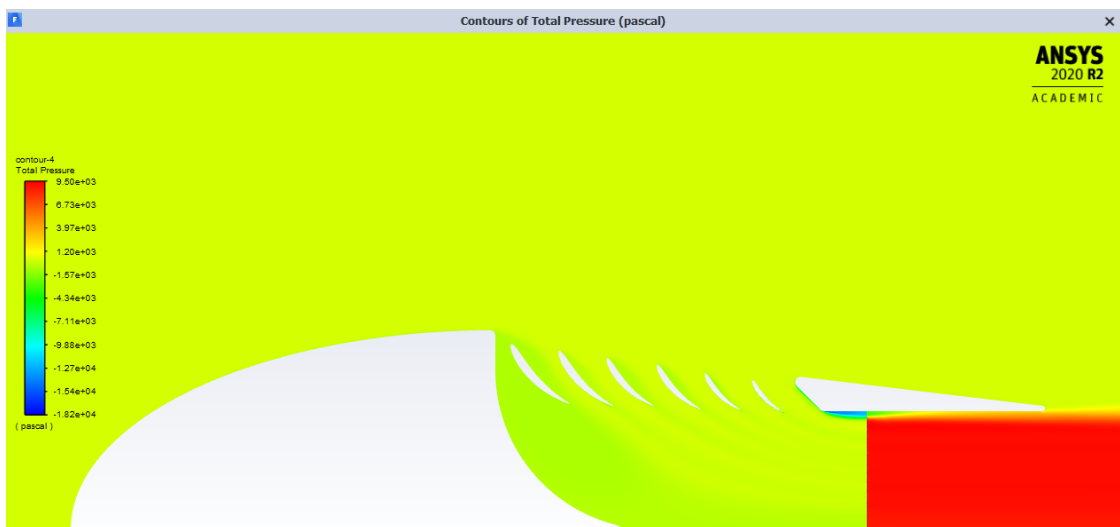
Figure A.6: Contours of the total pressure for inlet velocity 20 m/s.
