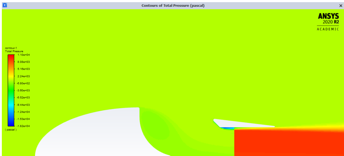
Figure B.2: Contours of the total pressure for inlet velocity 20 m/s.
