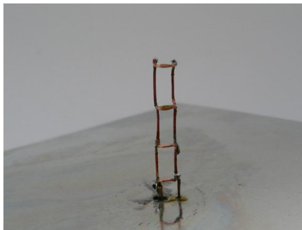
Fig. 3.2: Photograph of realized 4 loop antenna
