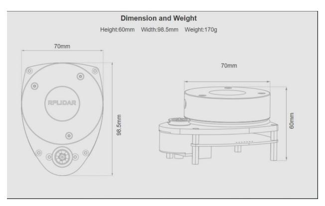
Figure 4 Dimensions of the RPLIDAR[25]
