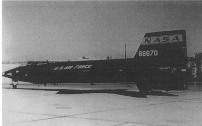
Fig. 7. X-15 rocket plane had on the exhaust nozzle coating made of Zirconia-calcia/NiCr which is the first use of Thermal Barrier Coating in flight with crew. [23]
