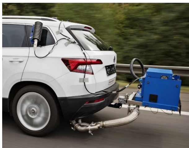
Figure 19: PEMS installed on a passenger vehicle [57]
