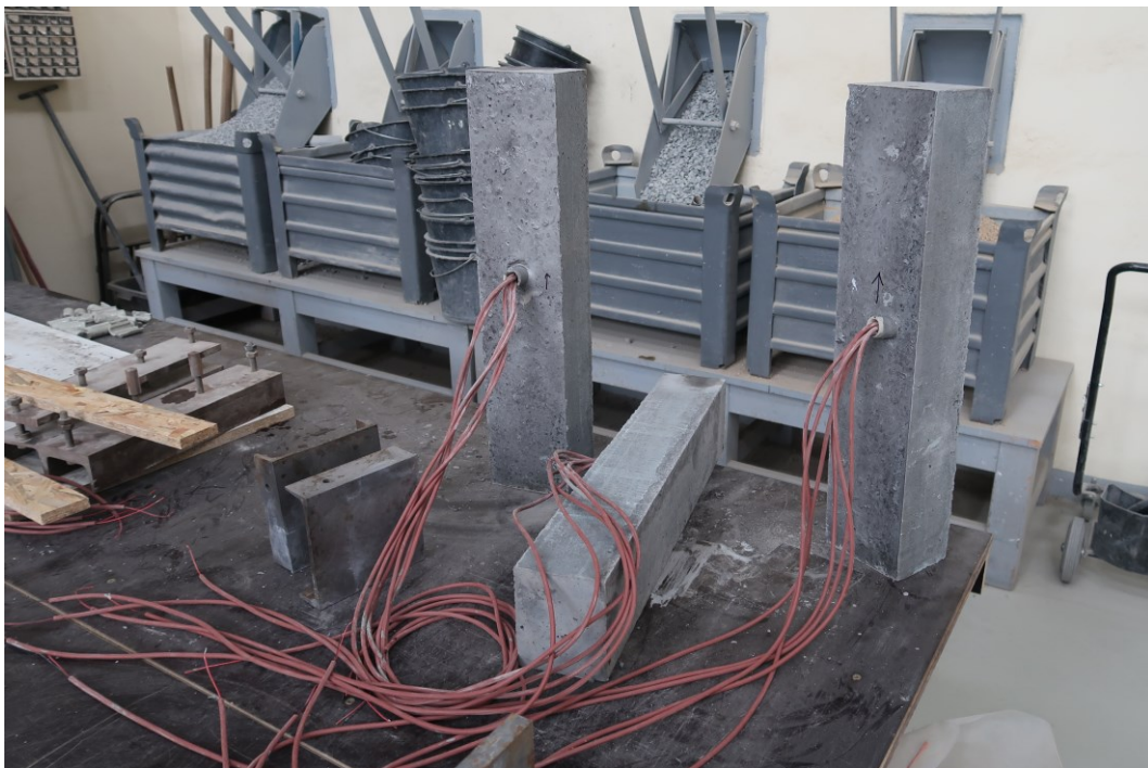
Figure 49 Finished concrete beams after concreting and cavern filling (might be seen on central beam, as darker stain on edge in back) (picture: J. Zatloukal)
