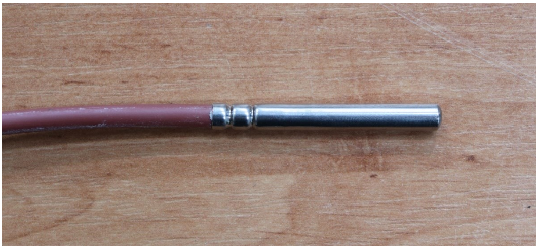
Figure 18 PT1000 Thermometer used in measurement system
