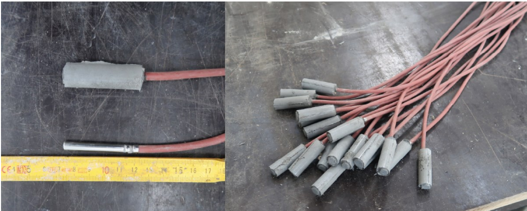
Figure 44 Finished thermometers suitable for insertion into casing beams (picture: J. Zatloukal)
