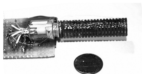
FIG. 3. The fluxgate gradiometer shown with 1-cent coin.
